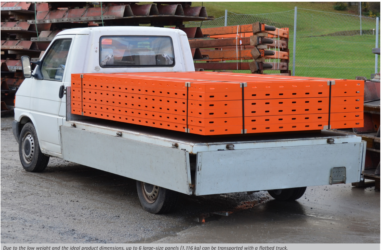
Due to the low weight and the ideal product dimensions, up to 6 large-size panels (1.116 kg) can be transported with a flatbed truck.
